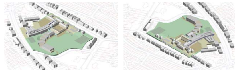
Massing studies The scale of the new building is sensitive to the existing buildings on site and surrounding conservation area. The building is centered to the site, pulled back from site boundaries to provide external teaching and playing spaces and avoid overlooking issues.
